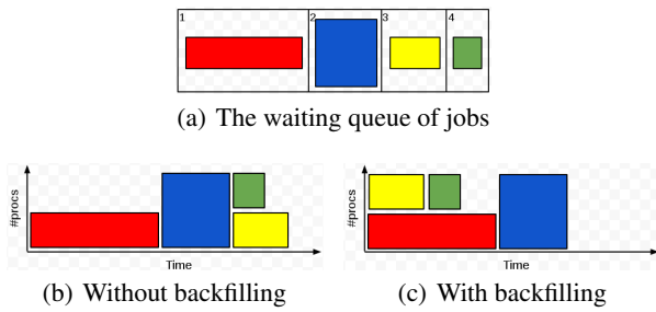
Figure 1: The backfilling mechanism
